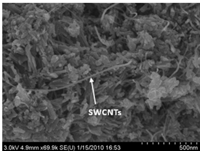
Figure 3. SEM images of the titania nanotube/SWCNT composite.
